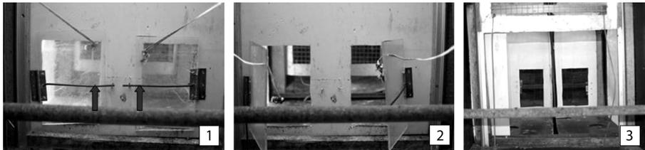
**Figure 2.** 1. The opening mechanism of the two Plexi-glass doors in the test compartment C. The two arrows mark the two levers that can be lifted to open either of the doors. 2. The doors in an opened state. Once the lever is lifted the door is pulled open by a stretched rubber ribbon. 3. View from the entrance into the 2 compartments of the middle chamber B, in which K and I were placed
